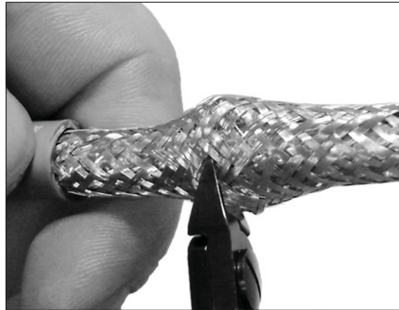
Figure 34 Cable Braid Bulge/Cutting
