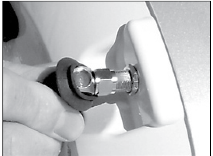
Figure 7: Connecting the Antenna Cable
