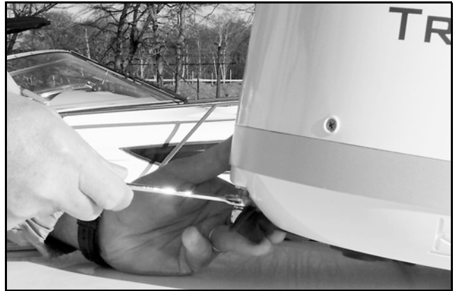
Figure 10: Connecting the Antenna Cable
