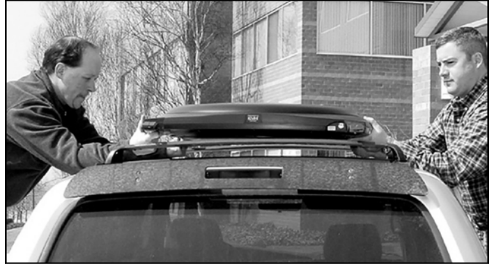
Figure 6: Placing the Antenna on the Crossbars
