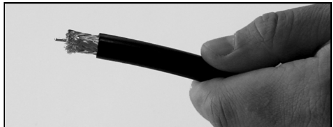
Figure 96: Cable Stripped, Exposing Dielectric
