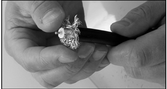
Figure 97: Flaring the Braid
