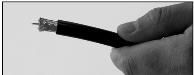
Figure 95: Cable Stripped, Exposing Dielectric
