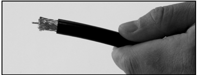
Figure 99: Cable Stripped, Exposing Dielectric
