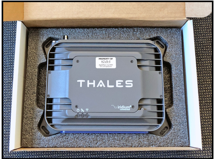
Figure 17: BDU Protective Foam
