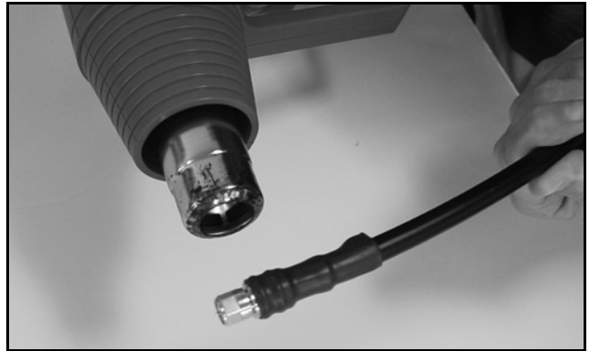
Figure 91: Applying the Heat Shrink Tubing
