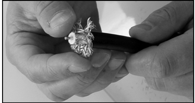
Figure 85: Flaring the Braid
