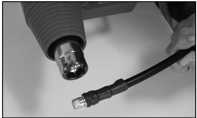
Figure 90: Applying the Heat Shrink Tubing
