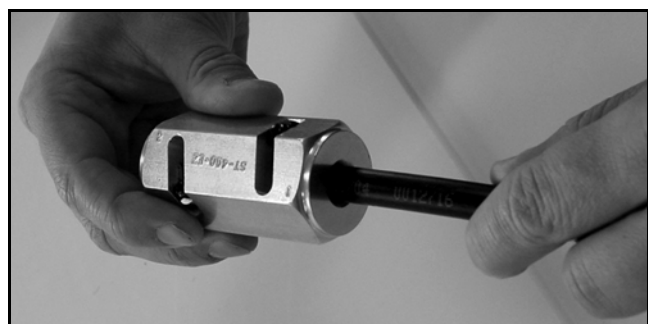
Figure 99: Stripping the End to Expose the Center Conductor
