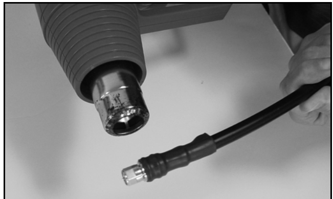
Figure 109: Applying the Heat Shrink Tubing
