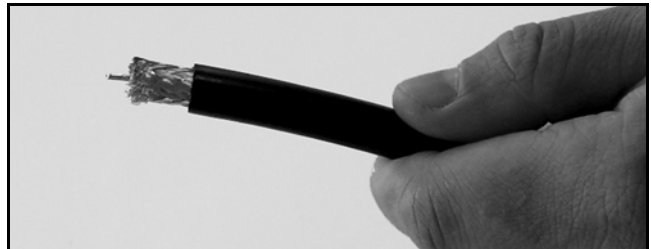
Figure 102: Cable Stripped, Exposing Dielectric
