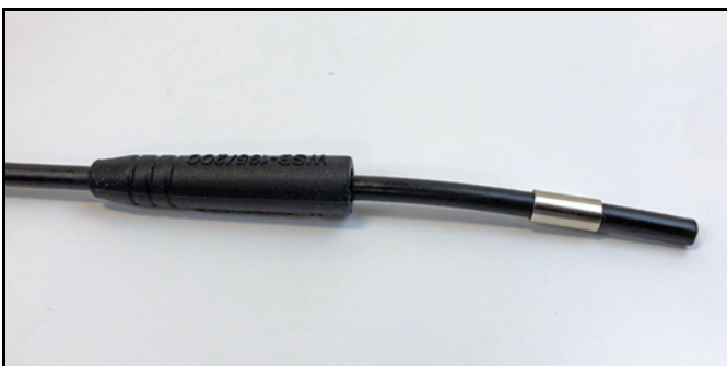
Figure 46: Placing the Rubber Boot and Ferrule onto the Cable
