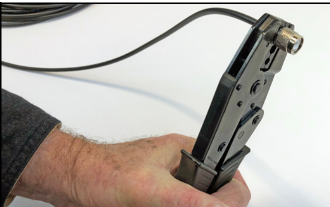
Figure 55: Crimping the Ferrule onto the Cable
