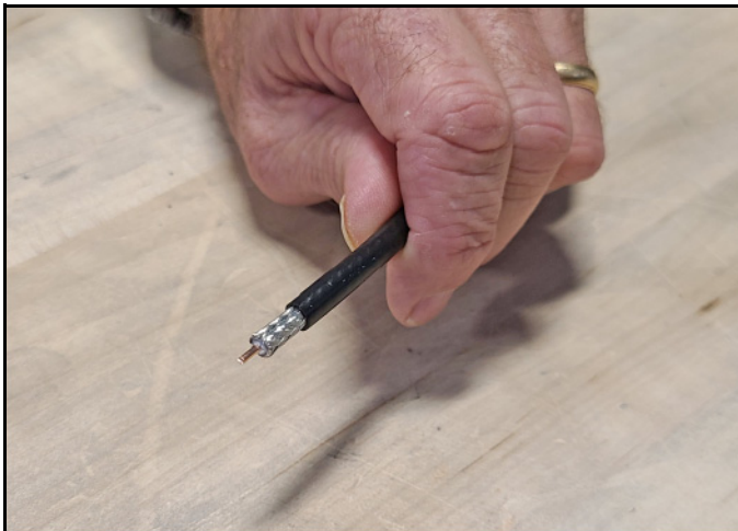
Figure 74: Cable Stripped, Exposing Dielectric
