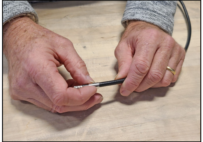
Figure 71: Placing the Ferrule
