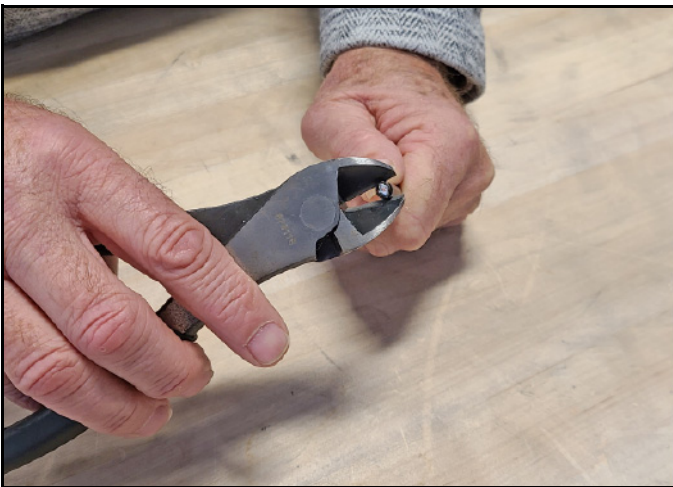
Figure 71: Reshaping the Cable
