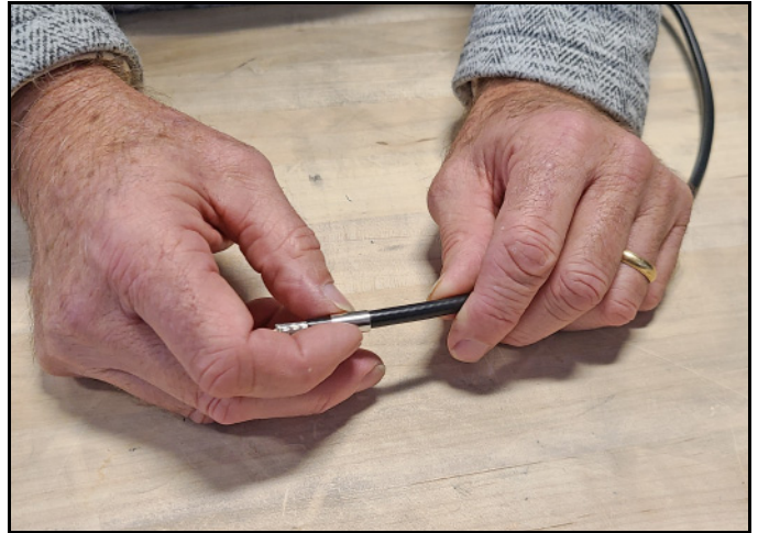
Figure 72: Placing the Ferrule
