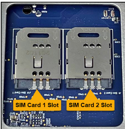
Figure 55: BDU SIM Card Slots
