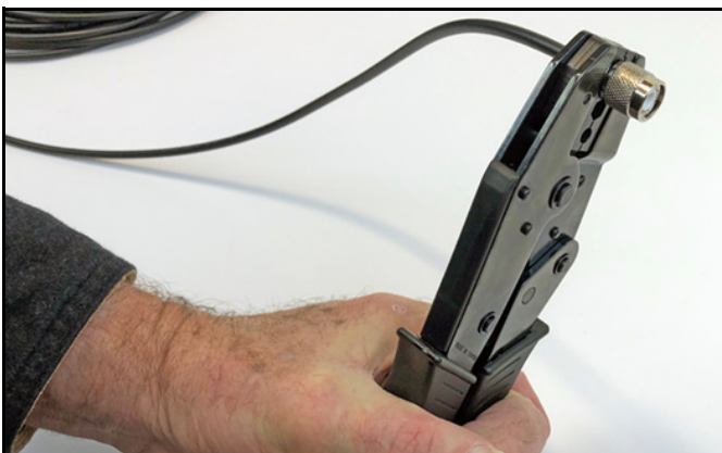
Figure 77: Crimping the Ferrule onto the Cable
