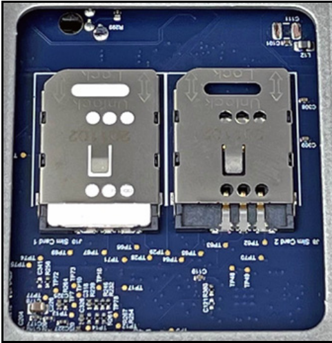
Figure 58: SIM Card Installed, Screen Locked in Place
