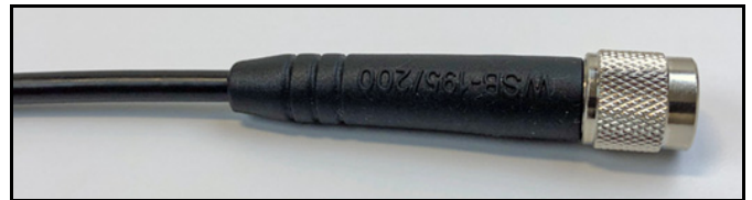
Figure 79: Rubber Boot in Place Over Ferrule
