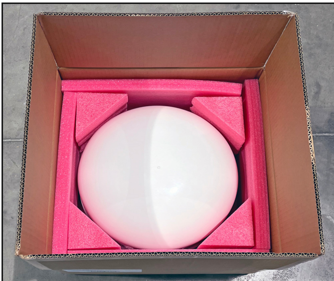
Figure 22: ADU Protected in Foam Base
