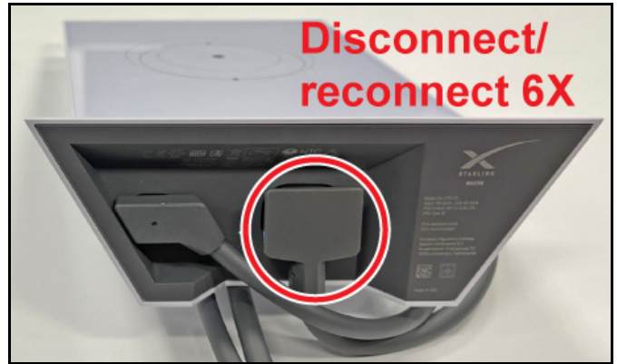
Figure 6: Starlink Gen 2 Router Power Cable Connection
