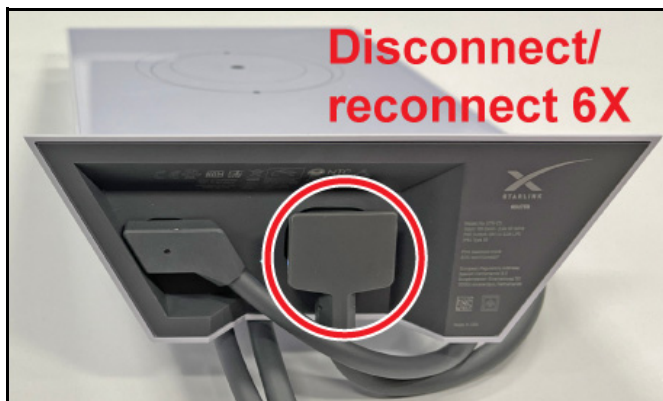
Figure 16: Starlink Gen 2 Router Power Cable Connection
