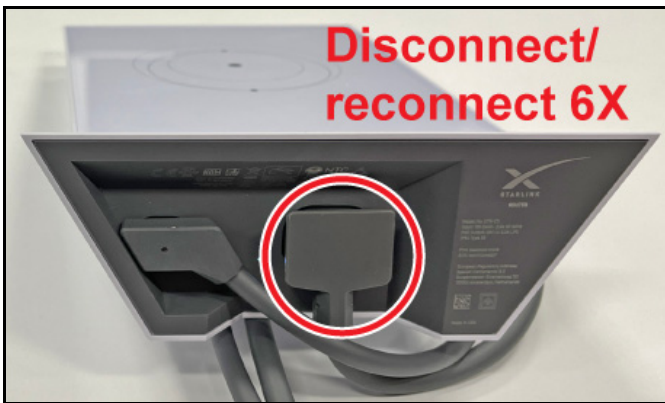
Figure 5: Starlink Gen 2 Router Power Cable Connection
