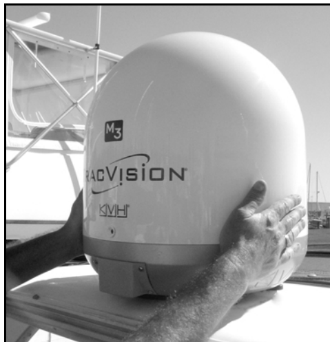
Figure 3 Removing the Radome
