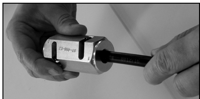
Figure 102: Stripping the End to Expose the Center Conductor
