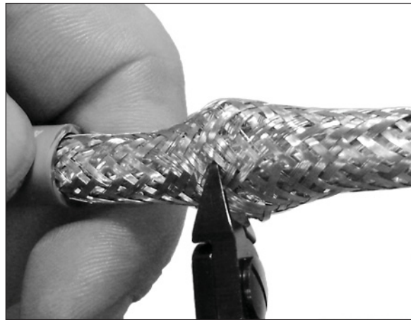
Figure 33: Cutting the Cable Braid Bulge
